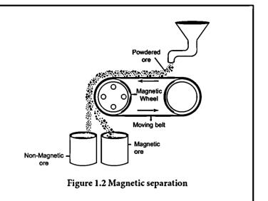
The magnetic part of the ore is attracted towards the magnet and falls as a heap close to the magnetic region while the nonmagnetic part falls away from it
